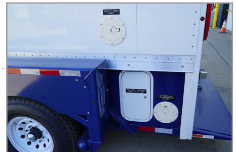
View of External Hookups
