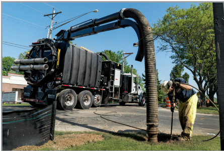
Porta Kleen's Hydro-Excavation truck on-site
