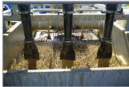
Slurry spraying onto the shaker deck
