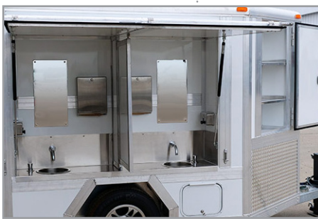
Divided handwash stations and storage cabinet.
