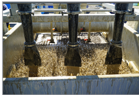
Slurry spraying onto the shaker deck
