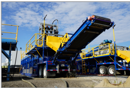
Sediment leaving the dewatering station
