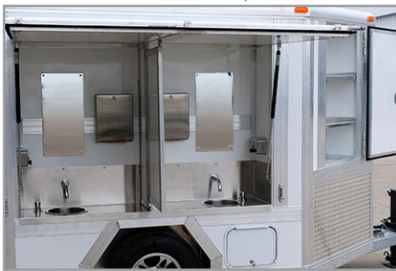
Divided handwash stations and storage cabinet.
