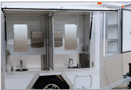
Divided handwash stations and storage cabinet.
